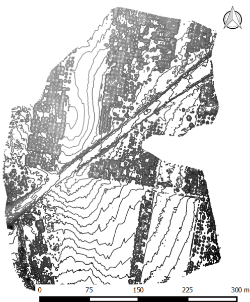
Figure 8: Contour lines (0.5 meter interval) generated from the photogrammetric digital terrain model.
