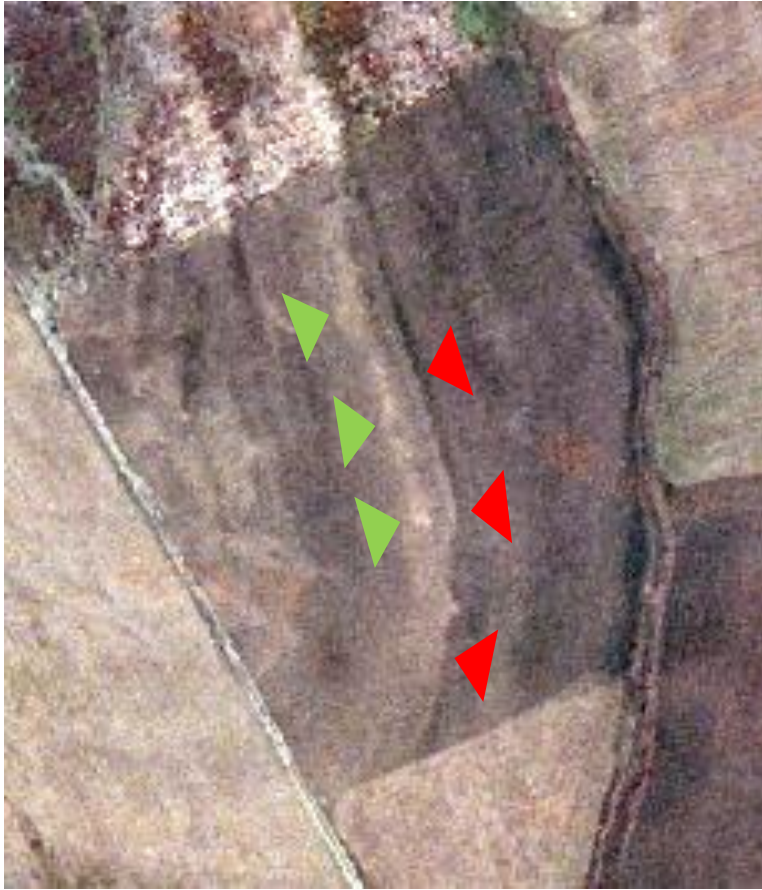
Figure 9: Example of possible coexistence of geological (lighter linear features, green arrows) and man-made features (sharpe linear darker line making a kind of an angle, see red arrows).
