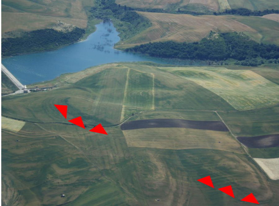
Figure 7: Linear features (some of which highlighted with red arrows) due to layered geology. Example of darker lines (due to different water retention of layers) from Southern Italy.
