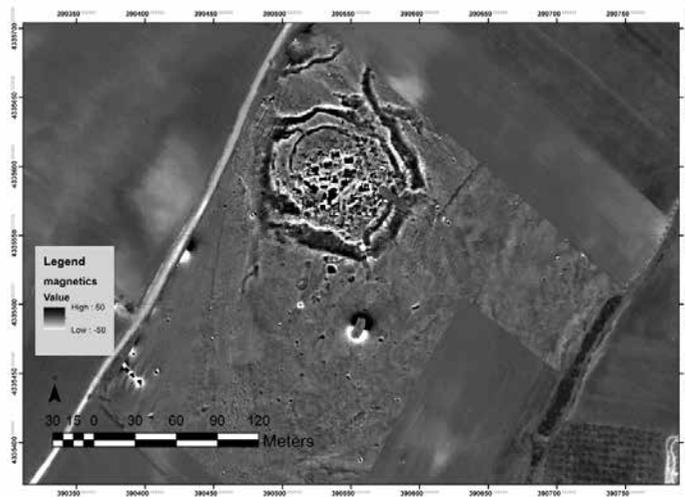
Fig. 1. Results of the SENSYS MX magnetic gradiometer survey at the Almyros 2 Neolithic tell
