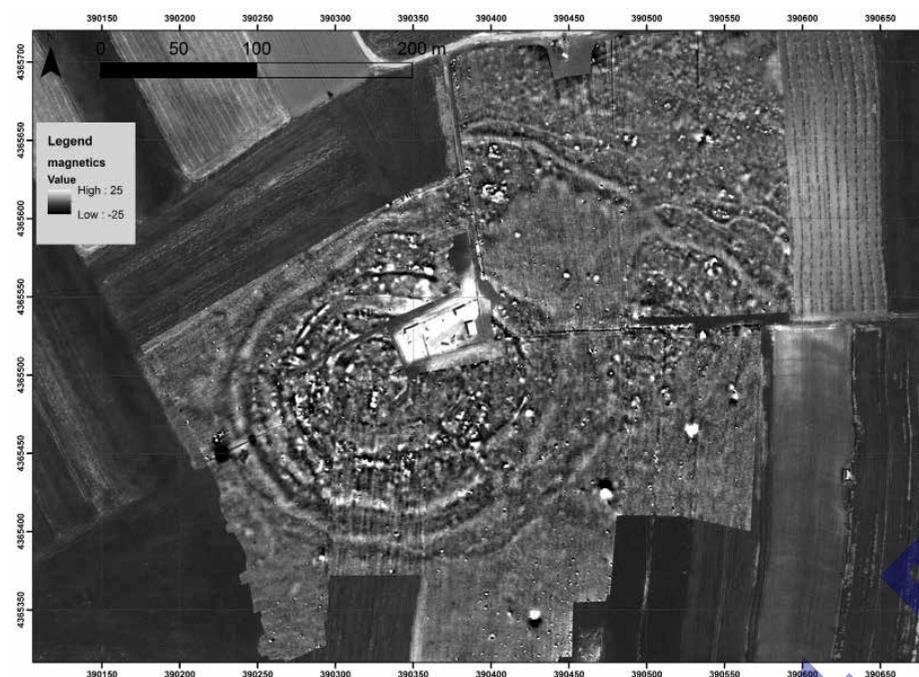
Fig. 3. *Magoula* Rizomilos 2. Results of the magnetic survey superimposed on a GeoEye-1 satellite image taken on May 4, 2010. The satellite image is a pansharpened Intensity-Hue-Saturation combination. A second smaller similar tell is suggested to the east of the settlement. To the north, the magnetic signature and the satellite data indicate traces of past flooding activity. According to the locals, the region used to be flooded regularly in historical periods.
